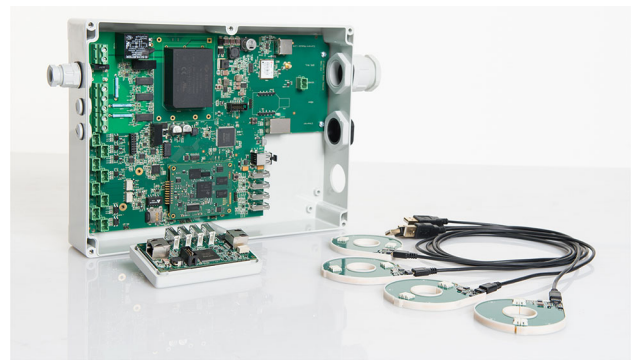
Fig. 1 GridBox base module, current module and Rogowski current sensors
