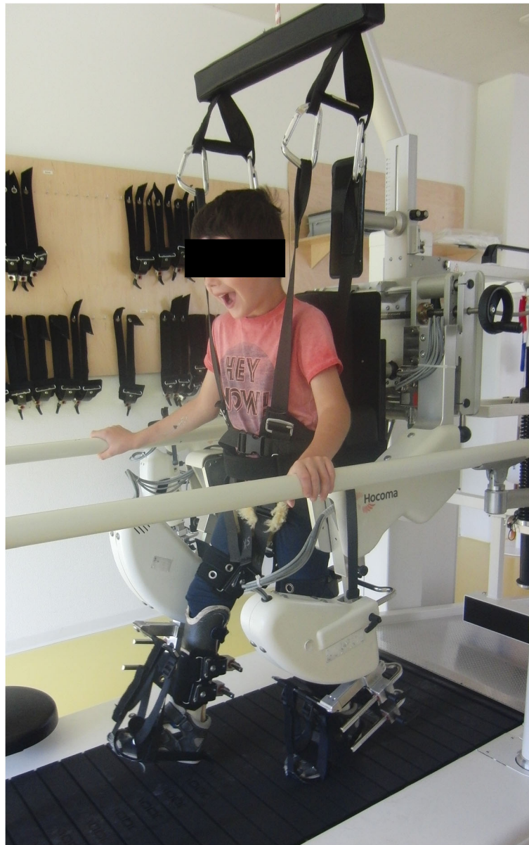
Fig. 1 Pediatric robot-assisted gait training with the Lokomat. The Lokomat automates gait therapy on a treadmill by two actuated leg orthoses, which can be individually adapted to the patient's legs and attached with three cuffs, while the patient is secured by means of a counter system with a harness providing partial body-weight support
