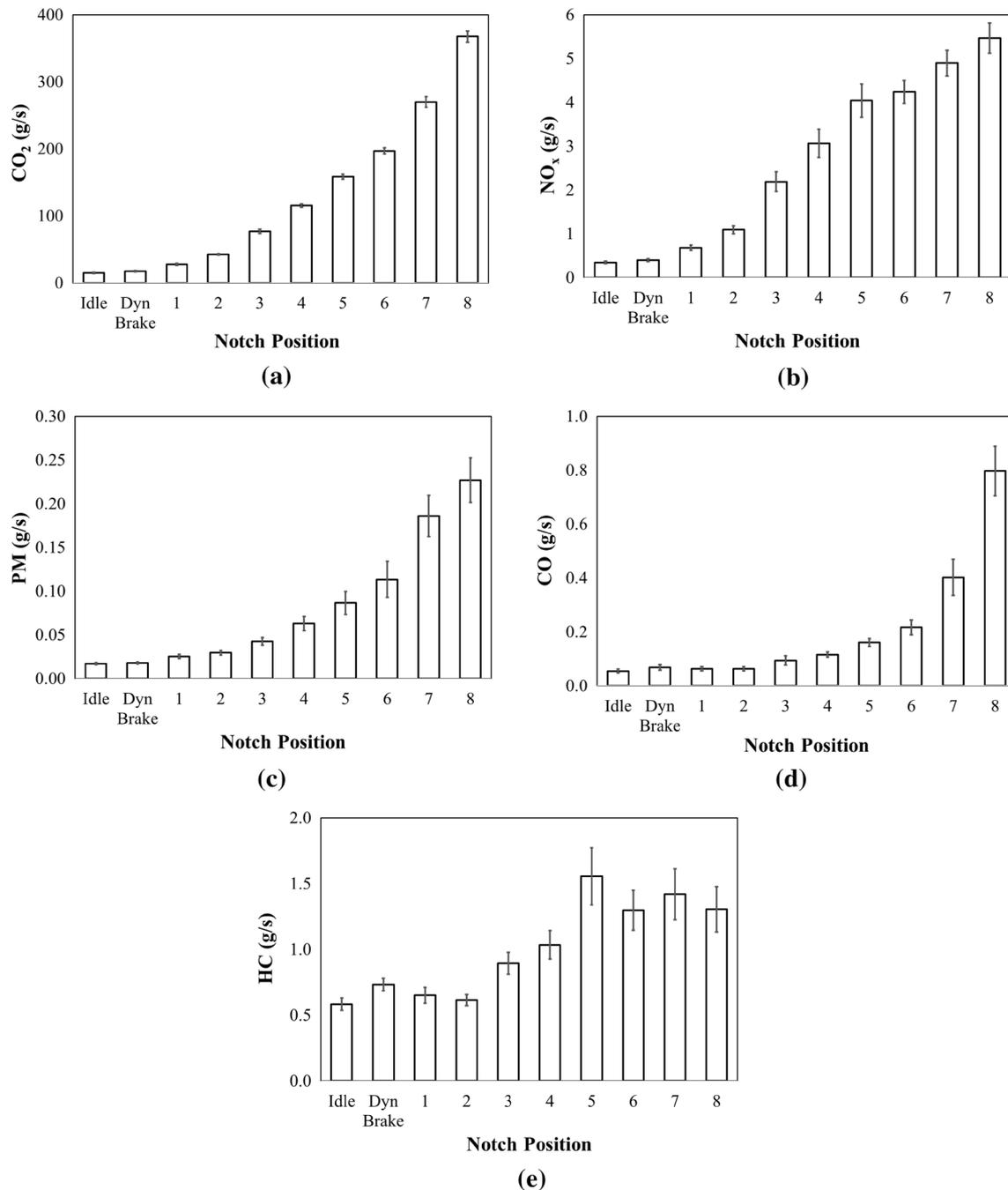
**Fig. 2** Fleet average emission factors of the prime mover engine at each notch position from thirty-six over-the-rail measurements using six locomotives. *Error bars* represent 95 % confidence intervals of the
