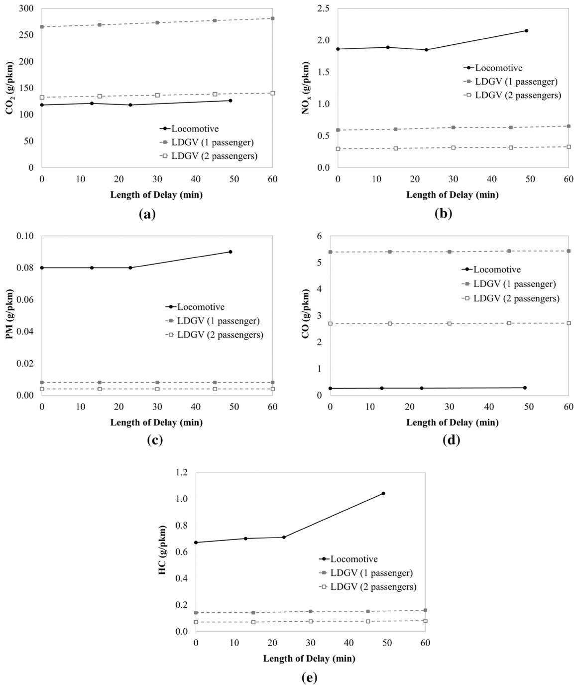
**Fig. 4** Fleet average locomotive and light-duty gasoline vehicle (LDGV) emission factors for on-time and delayed one-way trips between Raleigh and Charlotte, NC. **a** Carbon dioxide, **b** Nitrogen oxides, **c** Particulate matter, **d** Carbon monoxide, **e** Hydrocarbons
