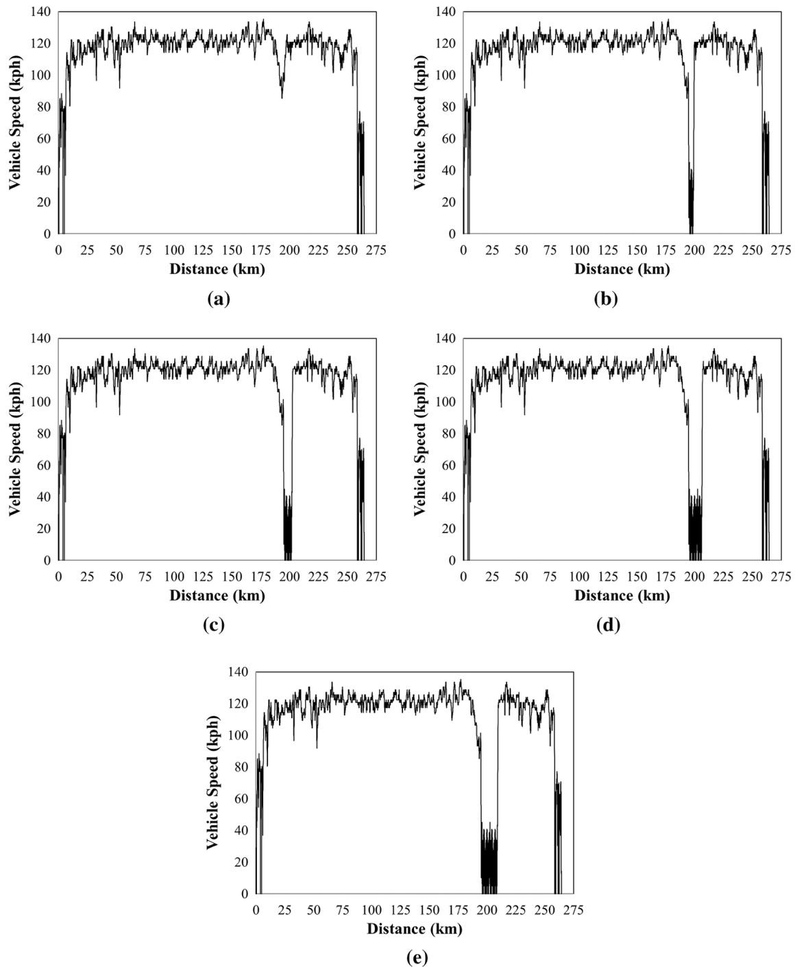
**Fig. 3** Highway vehicle drive schedules used in the Motor Vehicle Emissions Simulator (MOVES) software for on-time and delayed one-way trips between Raleigh and Charlotte, NC. **a** On-time, **b** 15 min delay, **c** 30 min delay, **d** 45 min delay, **e** 60 min delay
