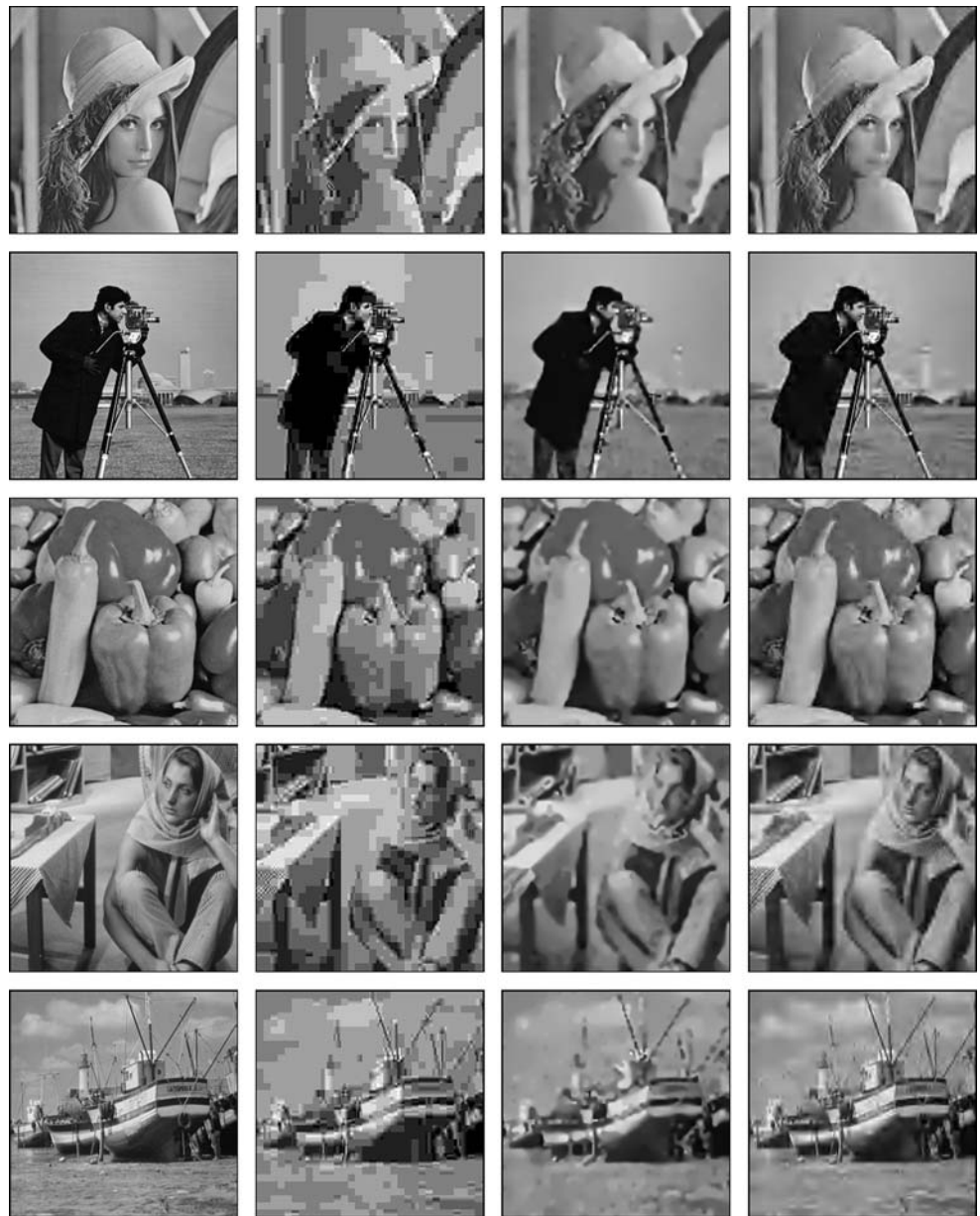
Fig. 9 Comparison of compression methods at 0.2 bpp for different test images (rescaled to 257 \times 257 pixels). Rows, top to bottom: lena , cameraman , peppers , barbara , boats . Columns, left to right: original image, reconstructed images after compression by JPEG, by EEDC, and by JPEG2000
