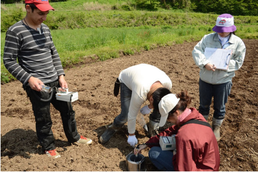
Measuring the surface dose of soil and space dose
