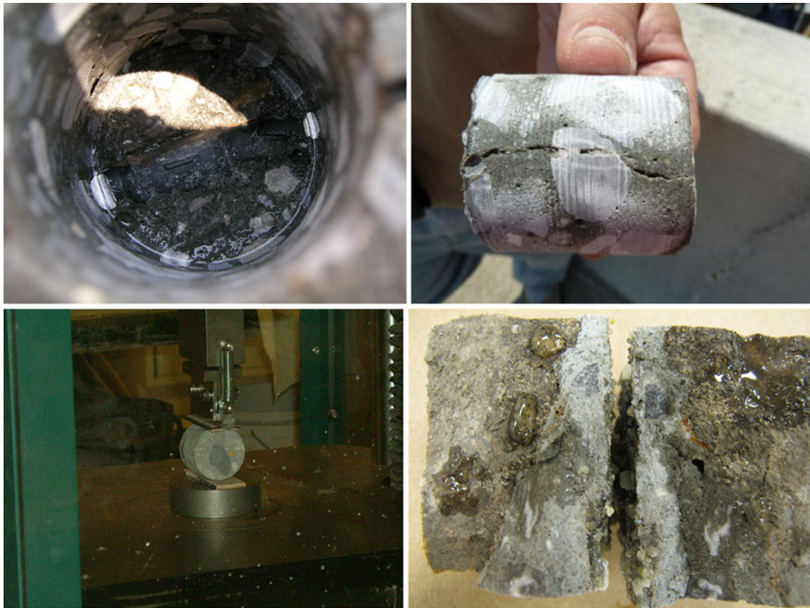
Fig. 5 Core removal, sampling, testing, and penetration.
