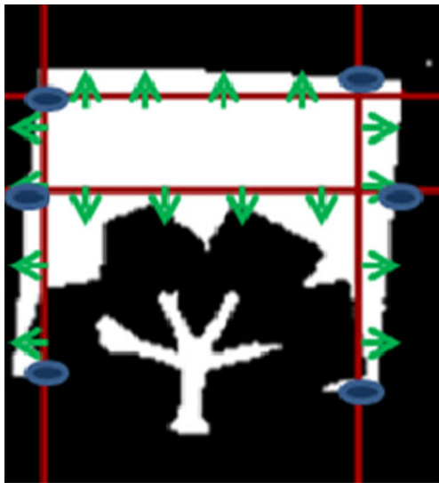
Fig. 7 Shows gradient points marked from each respective scan and stencil scan to define the edge. The blue circle represents a strong gradient point, G_i(x,y) , that forms a line segment cutting through patch. The green arrow represents the stencil scan direction to the approximate edge of the patch
