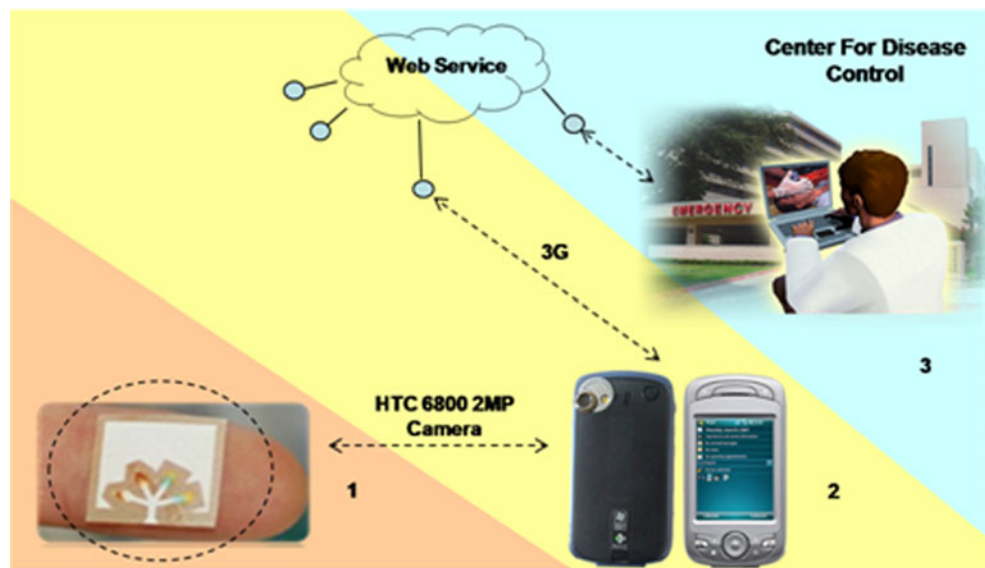
Fig. 1 Architectural overview of mobile dengue detection for 1) dengue template 2) embedded system platform 3) central server at Center for Disease Control
