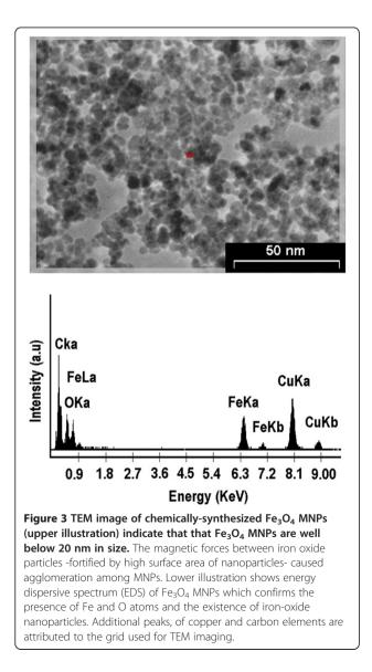
mentioned that additional peaks, belonging to copper and carbon element are attributed to the grid used for TEM imaging.
