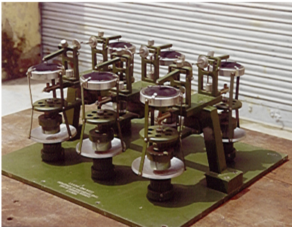
Fig. 25 Arrangement of a typical structural response recorder (photo: A. Mathur)
