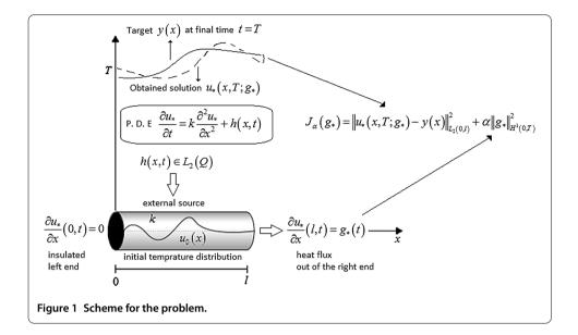
flux intensity function g(t) produces the heat distribution u(x, t; g) which is the solution of the PDE.
