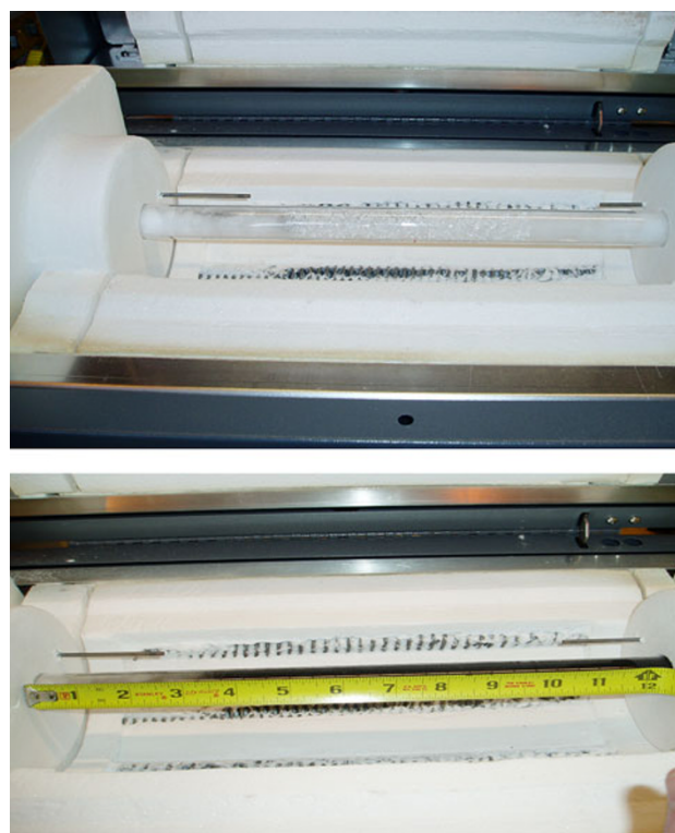
Fig. 5 Interior of the conventional electrical muffle furnace with reactor filled with quartz particles and quartz wool; top before reaction; bottom after carrying out an ethane-to-ethylene conversion process
