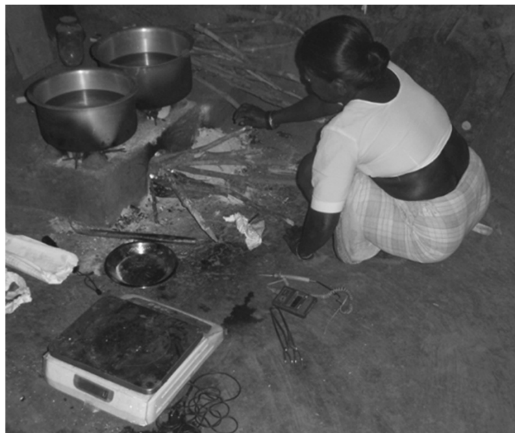
Figure 4 A woman firing cookstove in a two-pot water boiling test. Water boiling tests in the village were carried out with women, where a woman who cooks food fired her cookstove to find out its performance.
