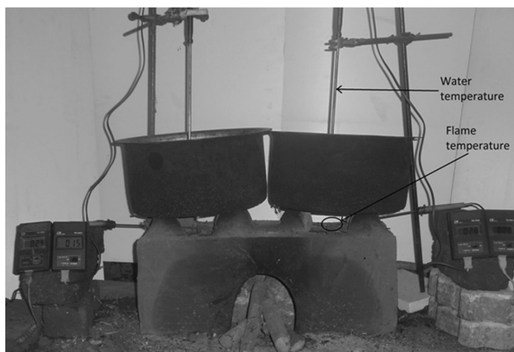
Figure 7 Experimental set-up to carry two-pot WBT in the laboratory. This shows the experimental set-up that was used to carry out the laboratory WBTs. Four thermocouples were used to measure the temperature of water and flame for both the pots and hearths.
