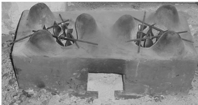
Figure 6 Twisted tapes hanging in the hearth holes. This shows the way to hang the twisted tapes in the hearth holes by using steel rods. They are placed in a way that they cover the cross-section of the hearth evenly.
