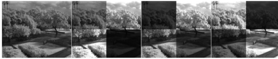
Figure 4 Gray-level images with non-homogeneous illumination variation. The 1st image is the raw infrared image, and the rest are the synthetic images.
