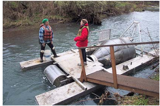
Fig. 4 Rotary screw traps used to collect emigrating salmonid smolts can be used to collect juvenile lamprey and provide information on the distribution of spawning and rearing areas. Photo by James P. Reed
