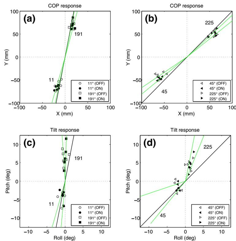
**Figure 6 Peak COP and tilt excursions for non-cardinal perturbation directions.** Mean values are shown for each subject with the display off (open symbol) and on (filled symbol). Green lines indicate 95% confidence intervals of the mean angles ( $A_{COP}$  and  $A_{phi}$ ) for each direction and black lines mark the directions of platform motion.
