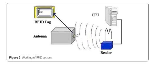
storing the data during transponder interrogation and response (Dimitriou 2005). The data consists of: (a) a unique identifier, (b) an operating system, (c) data storage (volatile/non-volatile), and (d) an EPC.
