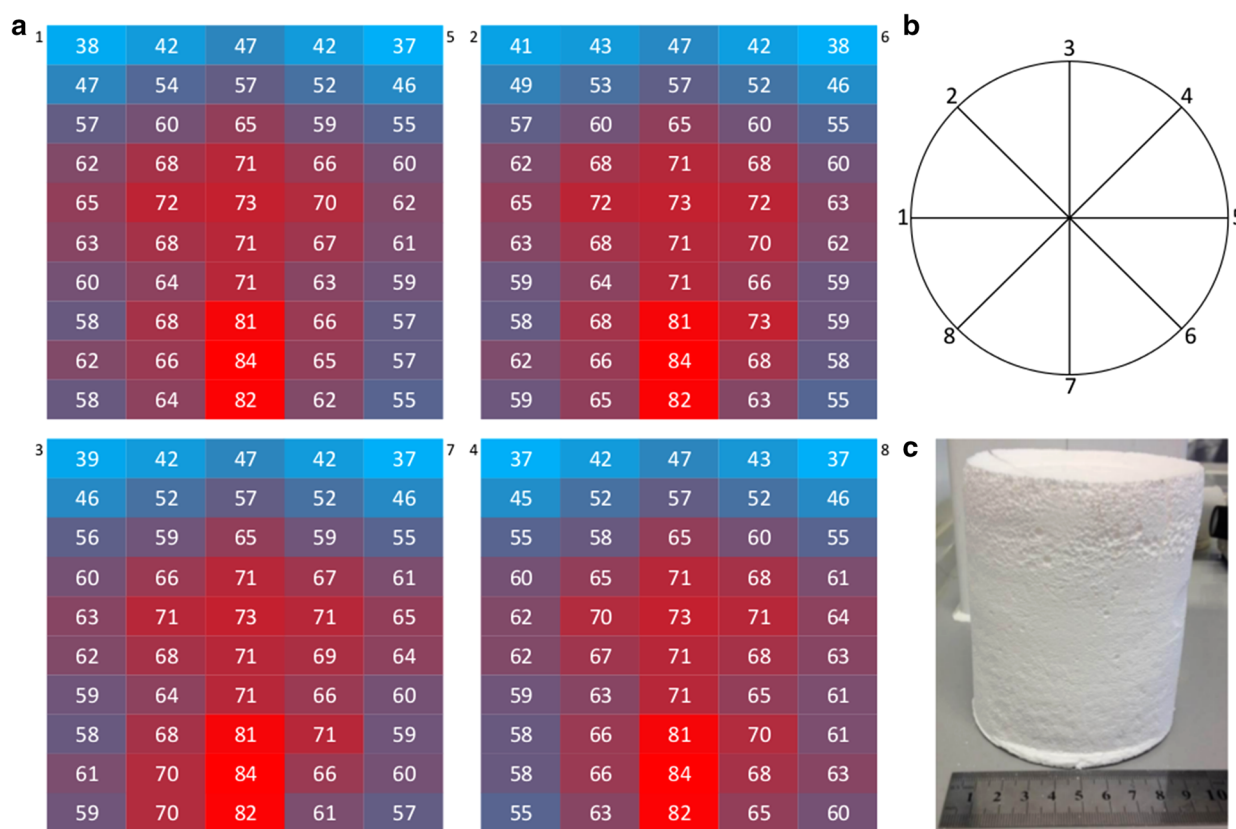
Fig. 8 Temperature profile inside a foam exposed to vent-like conditions. The temperature graphs present axial profiles based on the division of the foam as shown (1–5, 2–6, 3–7, 4–8) in the circle diagram ( inset ). Fluid at 70 °C was flowing into the foam at a rate of 15 mL/h with a coolant fluid at 20 °C being pumped into the reactor
