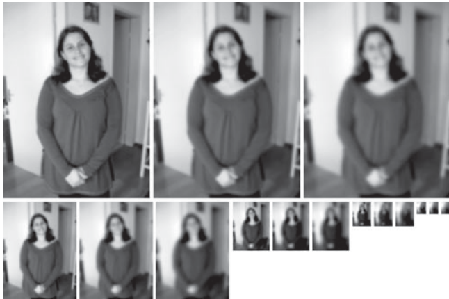
Figure 3. Example of a scale-space before the DoG computation.
