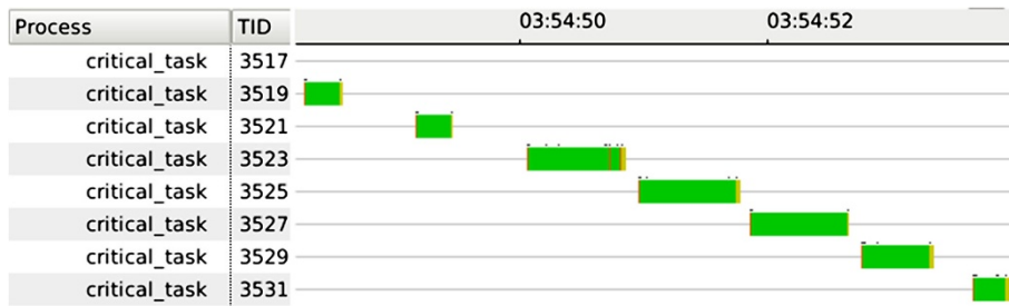
Figure 10 Execution of a periodic task as perceived by the VM. In some cases, the execution inexplicably takes longer to compute although the task appears as running.
