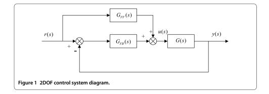
The transfer function of the entire 2DOF control system  $G_{2DOF}(s)$  from the reference signal r(s) to actual outputs y(s), is given by
