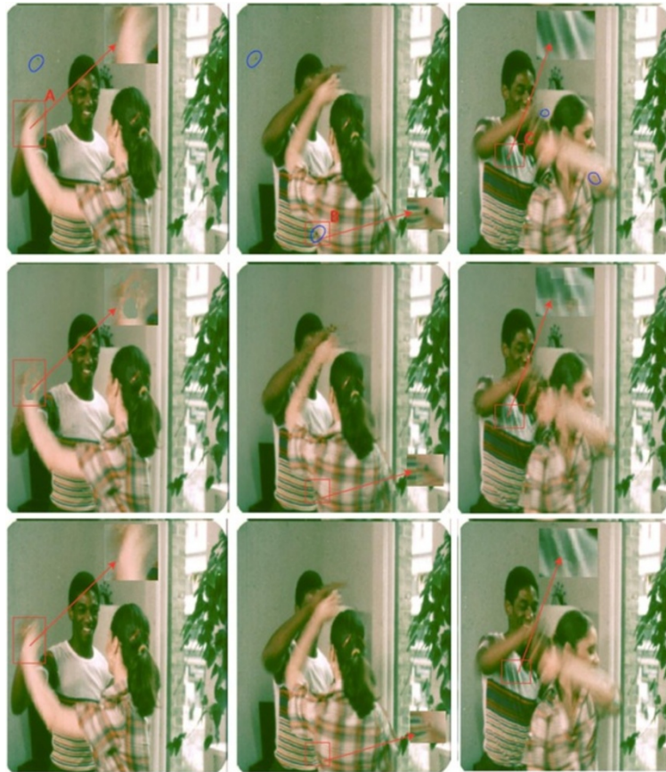
Figure 7 Frames 66, 70 and 77 of DanceB1 (top) with their reconstructions using JONDI (middle) and BTBR-F (bottom). Both systems perform well in removing blotches (shown in blue); however, JONDI could fail in removing blotches that lie near dark regions (box B). In addition, JONDI often misclassifies clean regions as corrupted. This could lead to severe reconstruction errors as shown in boxes A and C. On the other hand, BTBR-F classifies clean regions as uncorrupted, therefore disregard them from reconstruction.
