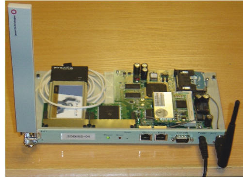
FIGURE 2: MeshDVBox: our wireless mesh router.
