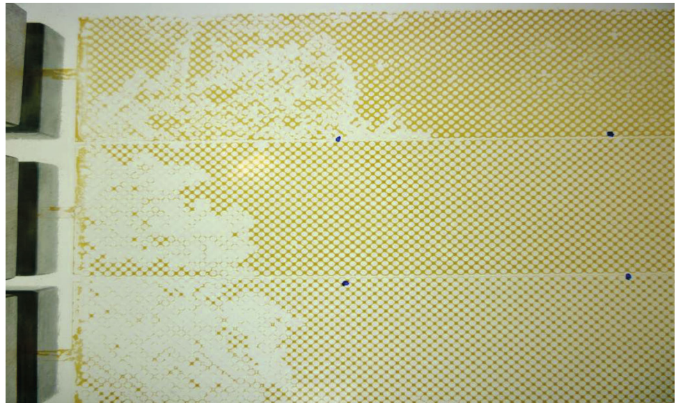
Fig. 11 Viscous fingering phenomenon in glass micromodel at time 2 (30 s) for 4.3 cP oil and 0.1 ml/min injection rate. The brown color represents oil, originally filling pore bodies and pore throats, while the white color represents both water and gains
