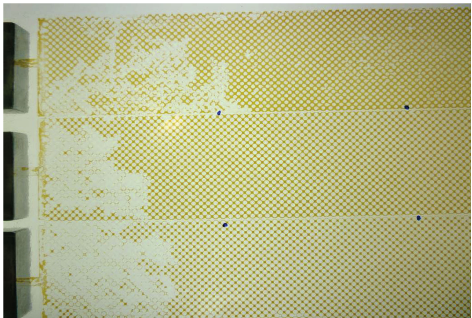
Fig. 10 Viscous fingering phenomenon in glass micromodel at time 1 (15 s) for 4.3 cP oil and 0.1 ml/min injection rate. The brown color represents oil, originally filling pore bodies and pore throats, while the white color represents both water and gains
