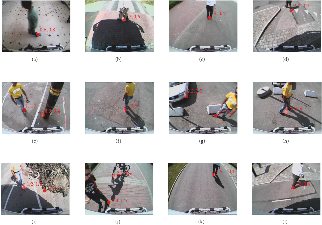
FIGURE 12: Result images showing typical algorithm output. A red dot shows the closest point of contact of each obstacle with the ground.
