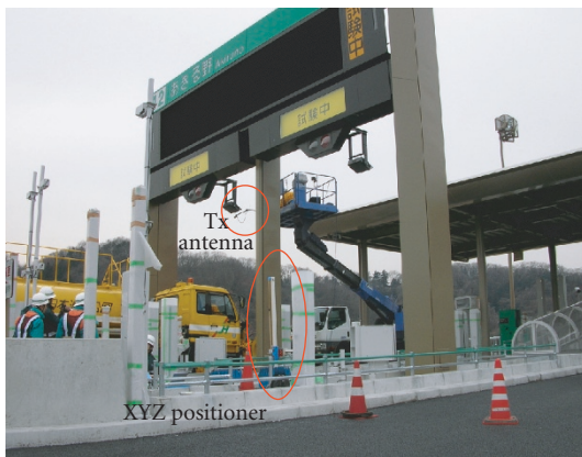
FIGURE 2: Previous measurement at ETC gate; it generally required to close the toll gates.
