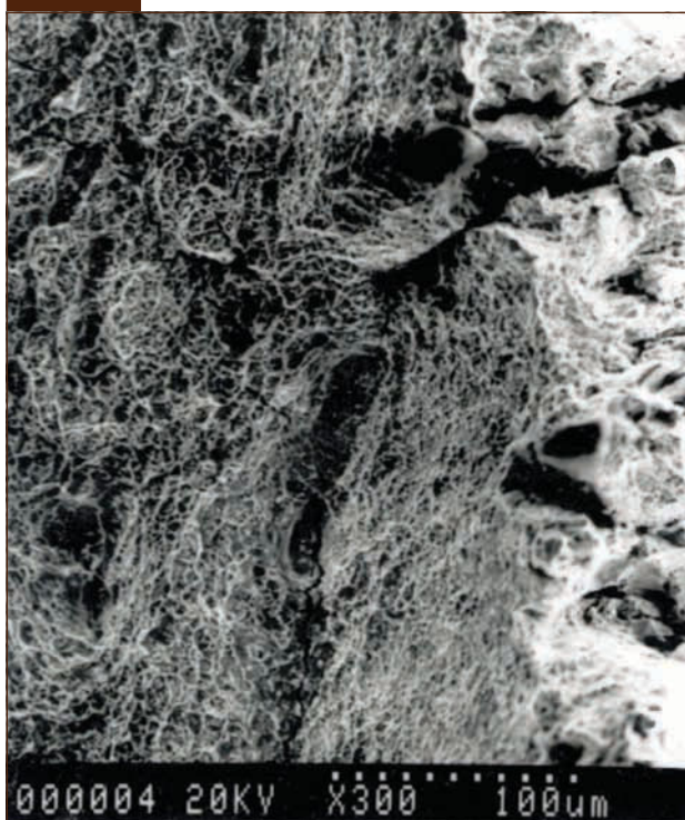
SEM image of the fracture surface of sample 4 after immersion in an aqueous 10 % \text{FeCl}_3 solution
