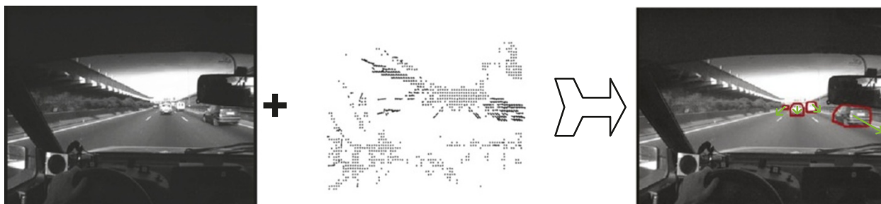
Figure 1 Joining of static and dynamic results to identify image objects.
