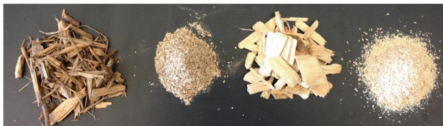
Figure 1 Biomass samples used in this study (from left to right) forestry residues (un-milled), forestry residues (2 mm-milled), Douglas-fir woodchips (un-milled) and Douglas-fir woodchips (2 mm-milled).
