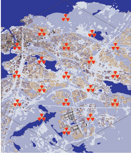
FIGURE 2: A 3-sectored hexagonal grid of 19 base stations with 2.0 km site spacing over the digital map. A 6-sectored configuration is formed based on 3-sectored antenna directions by adding antennas between the 3-sectored antennas. Traffic is distributed only inside the large hexagon.
