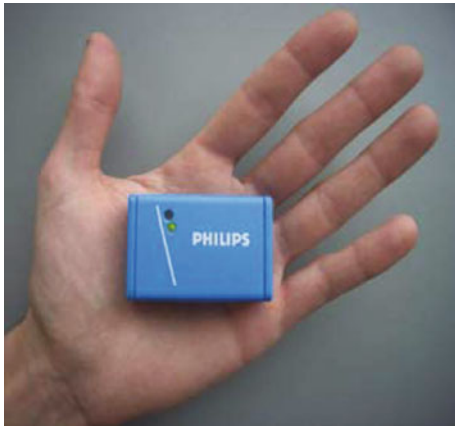
FIGURE 2. Inertial sensor unit. The wireless inertial sensor, which contains accelerometers, magnetometers, and gyroscopes. Note that for the current study only the data from the accelerometers and gyroscopes were used.
