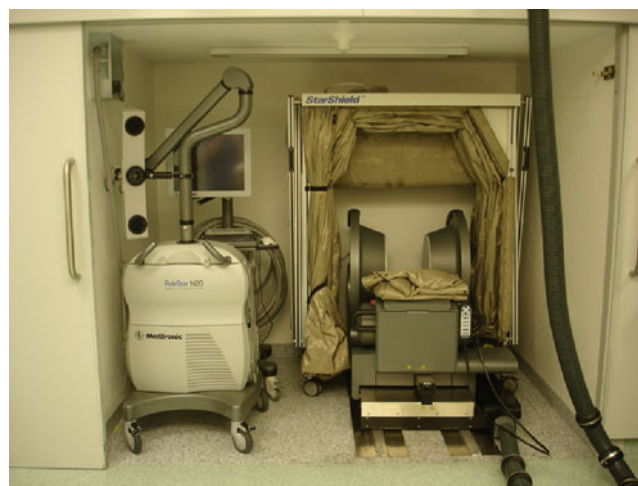
Fig. 1 PoleStar N20 system and StarShield® radiofrequency shielding
