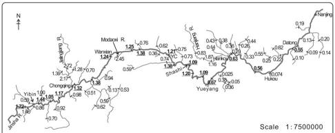
**Figure 3 Annual average silt concentrations (kg m^{-3}).** Concentrations in the main stream of the Yangtze River and its major tributaries in 1950 to 2000 (Wen 1999). Data in bold and without bold indicate the silt concentration in the main stream and in tributaries, respectively.
