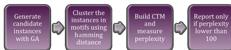
Fig. 2 Statistical GA algorithm workflow after including the use of topic models. This figure describes the updated flow of the Statistical GA algorithm after adding the perplexity measurement for the selection of solutions. There are four steps in this flow: the first one, in which the candidate instances are selected by the original Statistical GA; the second one, in which these instances are clustered attending to their similarity calculated by their hamming distance; the third one, which consists of building the CTM and measuring its perplexity, and the last step, which consists of reporting the motif if the perplexity calculated in the previous step is lower than 100
