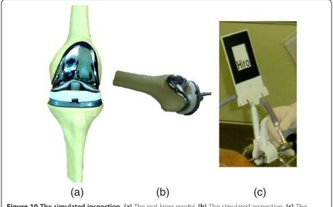
**Figure 10 The simulated inspection. (a)** The real knee model, **(b)** The simulated inspection, **(c)** The fiducial marker is fixed on the arthroscope.
