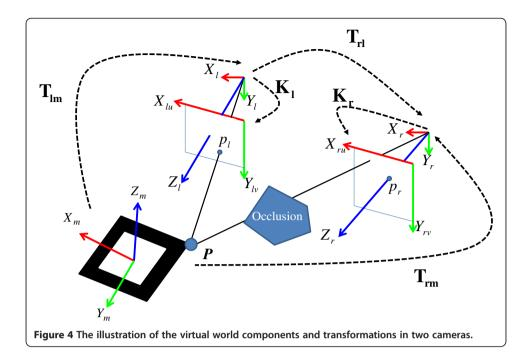
Given a 2D projection  $p_l$  on the viewing plane of the left tracking camera screen coordinates, its 3D point  $P_l$  in the left tracking camera coordinates can be computed by  $K_l$ . Then, the  $T_{lm}^{-1}$  times  $P_l$  makes  $P_m$ . Once  $P_m$  is obtained, its 3D projection  $P_r$  in the right tracking camera coordinates can be computed by  $T_{rl}$ . Its 3D relation between  $P_l$  and  $P_r$  is given by
