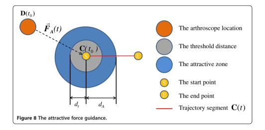
But when the arthroscope probe head comes between the sphere of radius  $d_t$  and  $d_A$ , the attractive force will be reduced linearly following Eq. (12).
