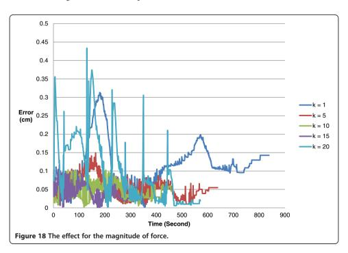
The force guidance is important to shorten the learning time. Hence, the magnitude of force has played an important role in the force guidance. The magnitude of force in this system can be adjusted by the simulated spring coefficient. Figure 18 indicates that the higher the spring coefficient, the better the learning result. However, unstable force will occur if the spring coefficient is set too high.
