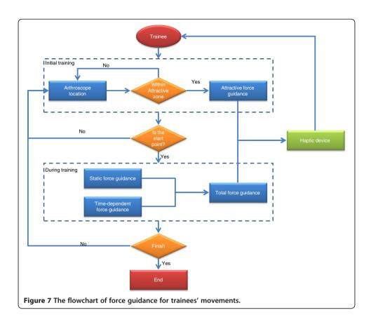
guiding forces including attractive force, static force and time-dependent force in the proposed simulator. The overall flowchart of the guiding force in the proposed simulation is illustrated in Figure 7.
