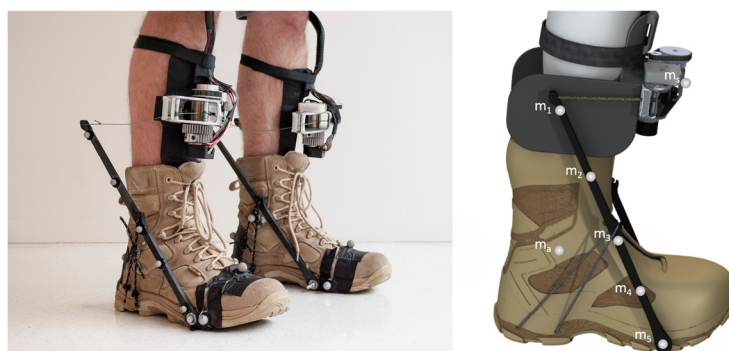
Fig. 1 Active autonomous ankle exoskeleton. The active autonomous ankle exoskeleton used a winch actuator on the shin to actuate the proximal ends of fiberglass struts attached to the boot. The winch actuator implemented a brushless DC motor and pulley transmission to wind a high strength cord. The motor controllers and batteries were worn around the chest and waist. Reflective markers on the strut were used to measure the deflection of the struts and the applied exoskeletal torque
