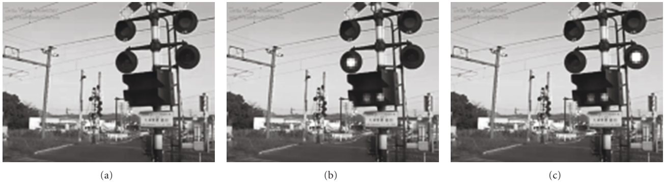
FIGURE 2: Background switches among several configurations controlled by the status of traffic lights.
