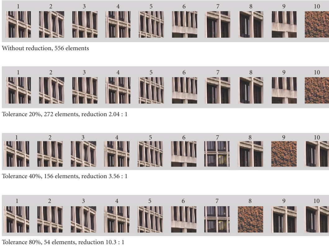
FIGURE 5: First 10 images objectively closest to a query (left) after applying feature vector reduction of prescribed tolerance.
