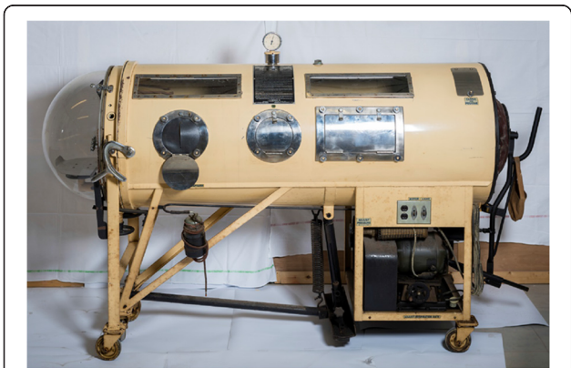
Fig. 1 The negative pressure ventilator (“Iron Lung”)
