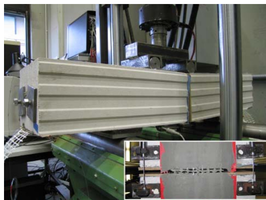
Fig. 18 Test setup with two-stone sample with sensor-textile on the bottom side (inclusion).
