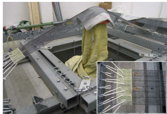
Fig. 16 Laboratory test in STFI e.V. in Chemnitz/Germany: forced deformation of a sensor-equipped geogrid and corresponding differential OTDR signal for different strain values.
