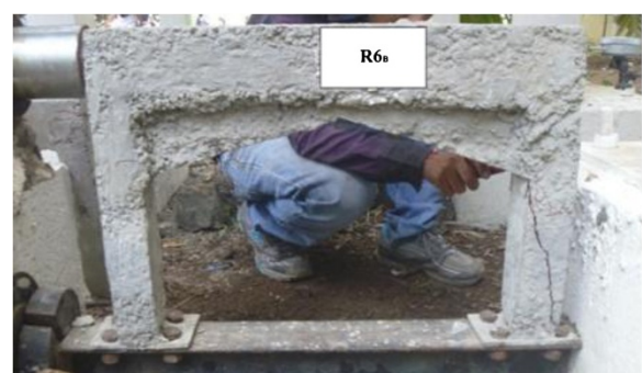
Figure 11 Central top bracing frame filled with concrete.
