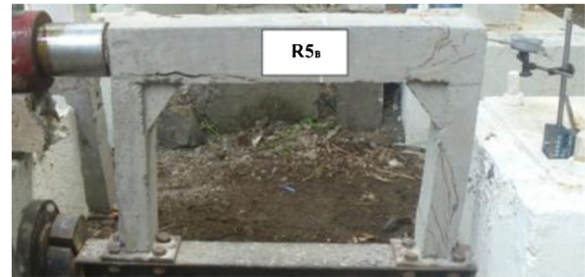
Figure 10 Corner top bracing frame filled with concrete.
