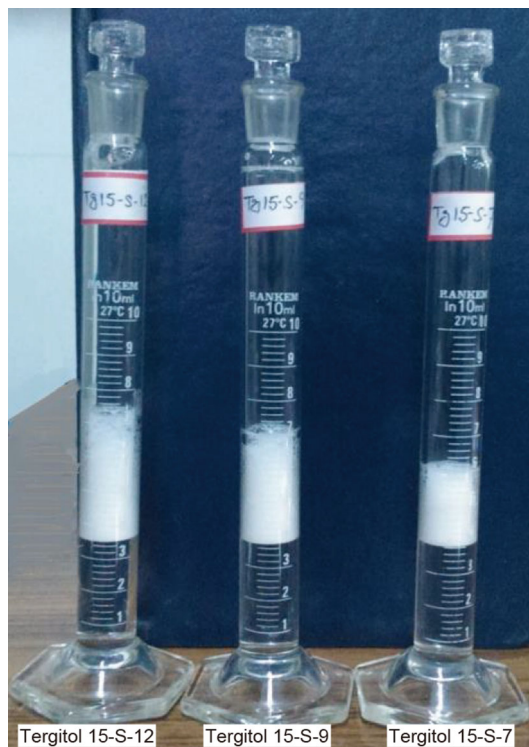
Fig. 6 Photograph of the foaming of the Tergitol surfactants in distilled water after several hours of equilibrium (from left to right: Tergitol 15-S-12, Tergitol 15-S-9, and Tergitol 15-S-7)
