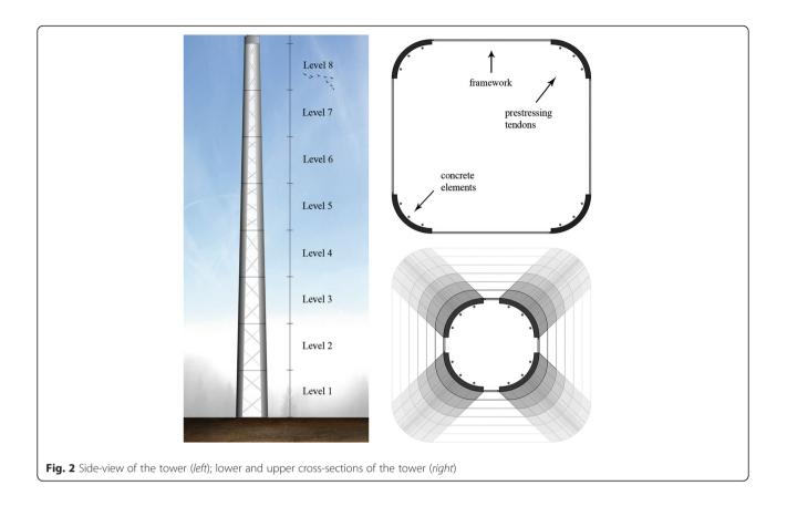
element is less than 20 t. This means that they can be delivered to the building site without the need for special transports, which are inevitably expensive.
