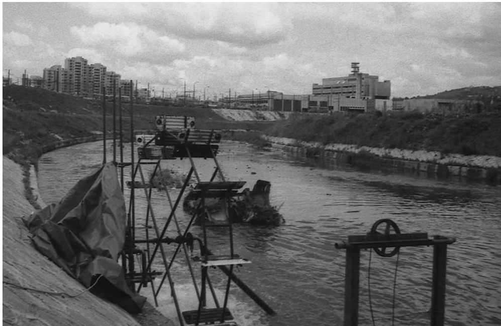
Figure 7. Water mill for generating electricity Photograph by Z. Kanlić, 15 September 1993. Reprinted with permission from Z. Kanlić.
