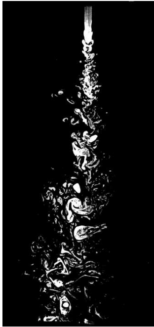
Figure 4: Turbulence as observed in a turbulent water jet (Van Dyke, 1982) reported in the book by Frisch (1995) (photograph by P. Dimotakis, R. Lye, and D. Papantoniu).
