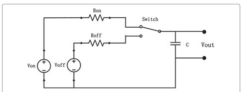
Figure 7 The RC circuit introduced by Azzam et al., where the voltage of capacitor C was used to simulate the HR and  $VO_2$  dynamics towards interval training protocols,  $V_{on}$ ,  $R_{on}$ ,  $V_{off}$ , and  $R_{off}$  are the onset and offset supplies and resistances respectively that were switched by a designed SPDT switch.
