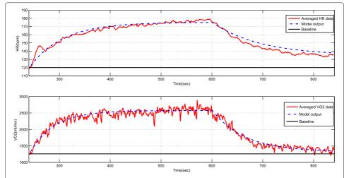
Figure 5 The model outputs vs. the averaged experimental data of HR and  $VO_2$  dynamics at onset and offset of exercise. The bold lines indicate the baseline of steady state level and closely reflect metabolic rates at warm-up. The red curves indicate HR and  $VO_2$  averaged data from experimental observations over twenty subjects. The dashed blue curves indicate the model outputs based on the determined parameters.
