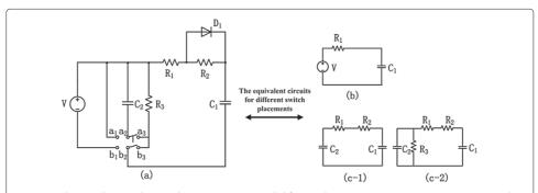
Figure 3 The single-supply switching RC circuit model for cardiorespiratory responses at onset and offset of exercise. (a). the proposed circuit model for both onset and offset of exercise; (b). the onset subcircuit; (c-1). the offset subcircuit c-1; (c-2). the offset subcircuit c-2.
