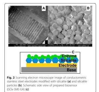
parameters. The procedure resulted in the formation of silicalite layer in the electrodes active zones (Fig. 2a).
