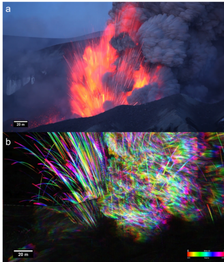
Figure 3 Image stacking was applied to identify and measure the trajectories of clasts. (a) The upper frame gives an impression of the number of particles ejected during a pulse (20 frames were stacked; this is essentially the picture that would have been created by a camera with an exposure time of 2/3 s). As this way of visualization only works at night and high contrast to a dark background, another standardized method was applied to track the trajectories: (b) 60 frames (i.e., 2 s of video footage) were stacked; the difference to each frame was calculated pixel by pixel and colored according to the respective frame. The image shows bent and straight trajectories, but only the latter were used for analysis. The visibility decreases on the right (downwind) side and is particularly low in the first quadrant (0° to 90°), as this sector is covered by ash clouds.
