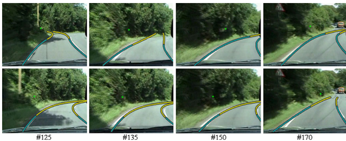
Fig. 12 Comparison of tracking performance with ( first row ) and without tracker switching ( second row )
