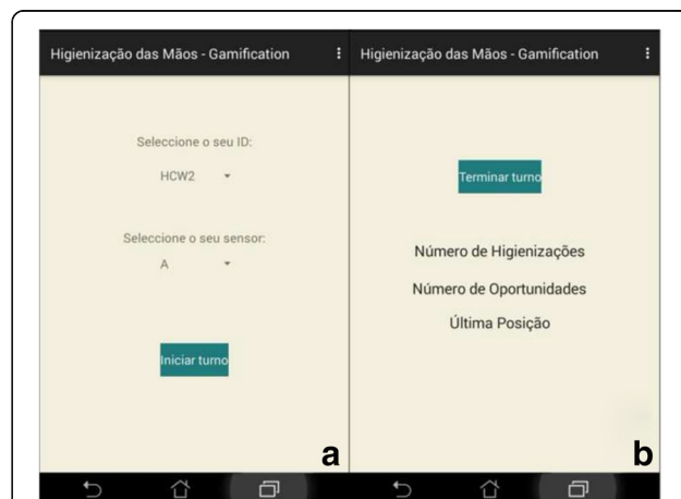
Fig. 4 Android App. a A screen for the HCW to select his/her ID and the ID of the sensor (s)he will be using. After clicking on the button, (s)he can start the shift; b The button allows a HCW to end the shift, thus the monitoring. Information is presented regarding the number of HH actions, number of HH opportunities and the last position where the HCW was detected, respectively
