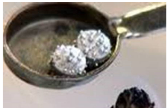
Fig. 1 Two tablets of copper amalgam in a spoon heated over an open flame ready to be crushed. With courtesy of the Norwegian TV Company NRK
